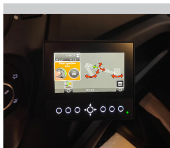
Outrigger setup from inside the cabin
